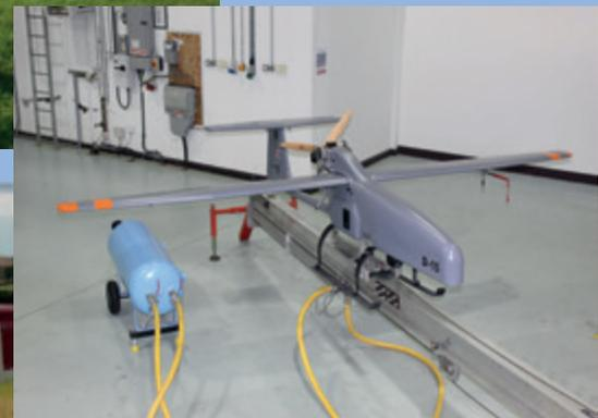
Launcher being filled with compressed air.
