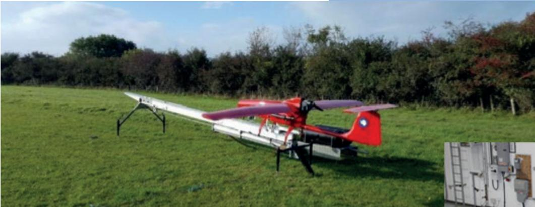
Dragon-15 used in conjunction with a compressed air inclined launcher
