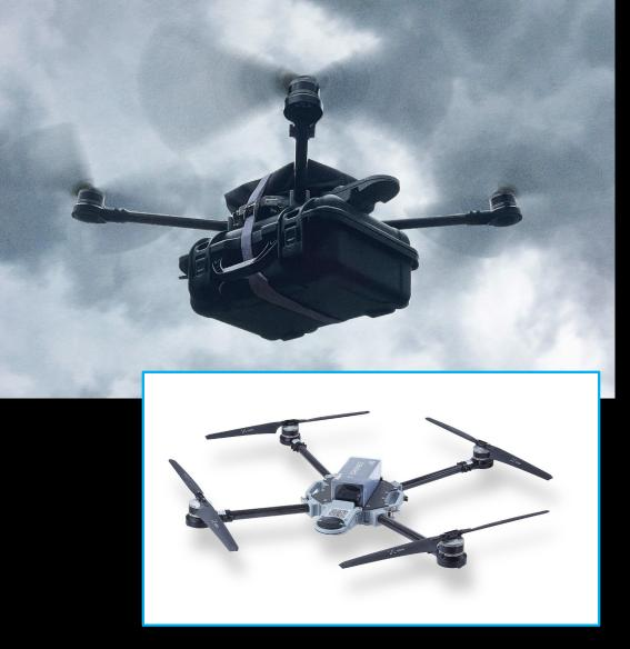
Flies with inertia navigation and radar – Does not use GPS, which can be jammed.
