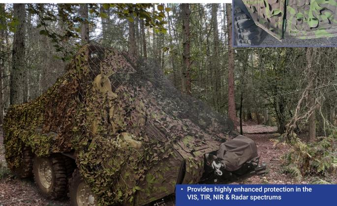
Can be combined with the Mk 7 3-D nets over the Mk 8 panels system.
