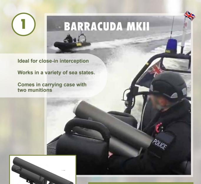
A hand-held device capable of launching a 30 metres arrestor line and two 3 ft (1metre) sea anchors.
