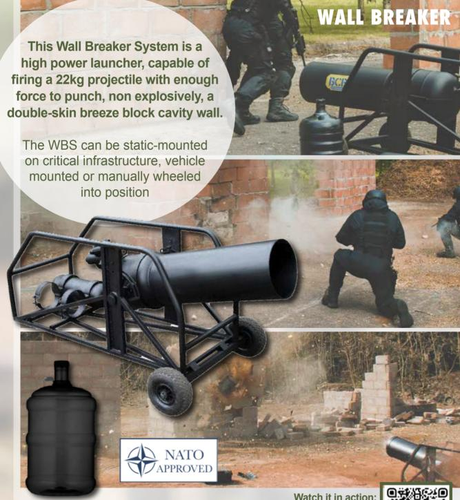
Fitted with a Recoil Mitigation System the WBS uses water or sand filled projectiles.
