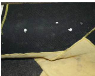
Zero trauma to femoral artery area following 5 kilo charge
