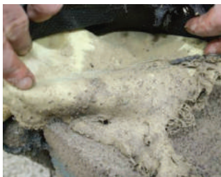
Fragmentation penetrated only 1 layer
