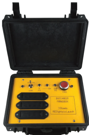
Control station for remote firing
