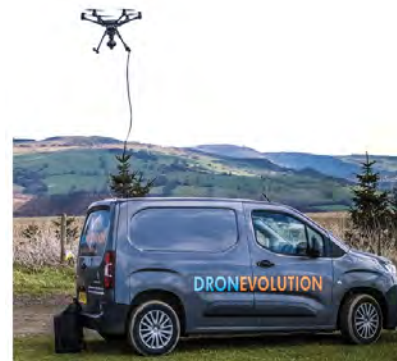
By powering the drone via a tether, attached to a ground station, the drone can stay in the air for extended periods of time.
