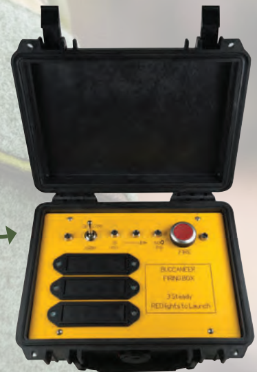
Control station for remote firing
