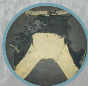
Result from 15kilo charge - Material still intact
