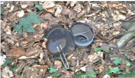
FireDragon – Cup base after burning 1 block of fuel
