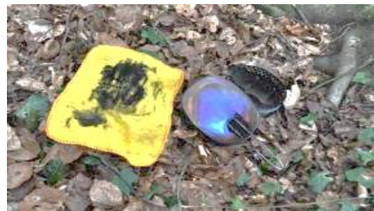
Methyl Esters competitor – Soot removed from base of cooker after burning 1 block of fuel.
