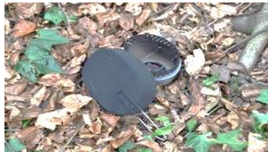
Methyl Esters competitor – Cup base after burning 1 block of fuel
