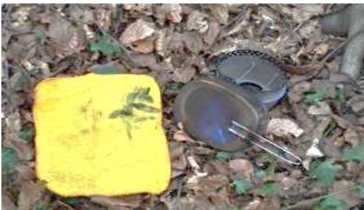
FireDragon – Soot removed from base of cooker after burning 1 block of fuel.
