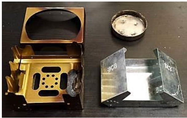
Standard Military Issue cooker (left) BCB Folding Cooker open to position 2 (right)
