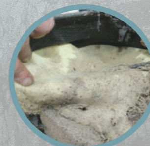
Fragmentation penetrated only 1 layer
