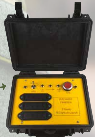
Control station for remote firing
