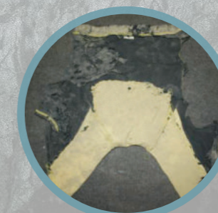
Result from 15kilo charge - Material still intact
