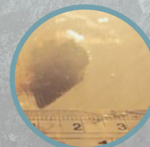
Ballistic gel with large fragment
